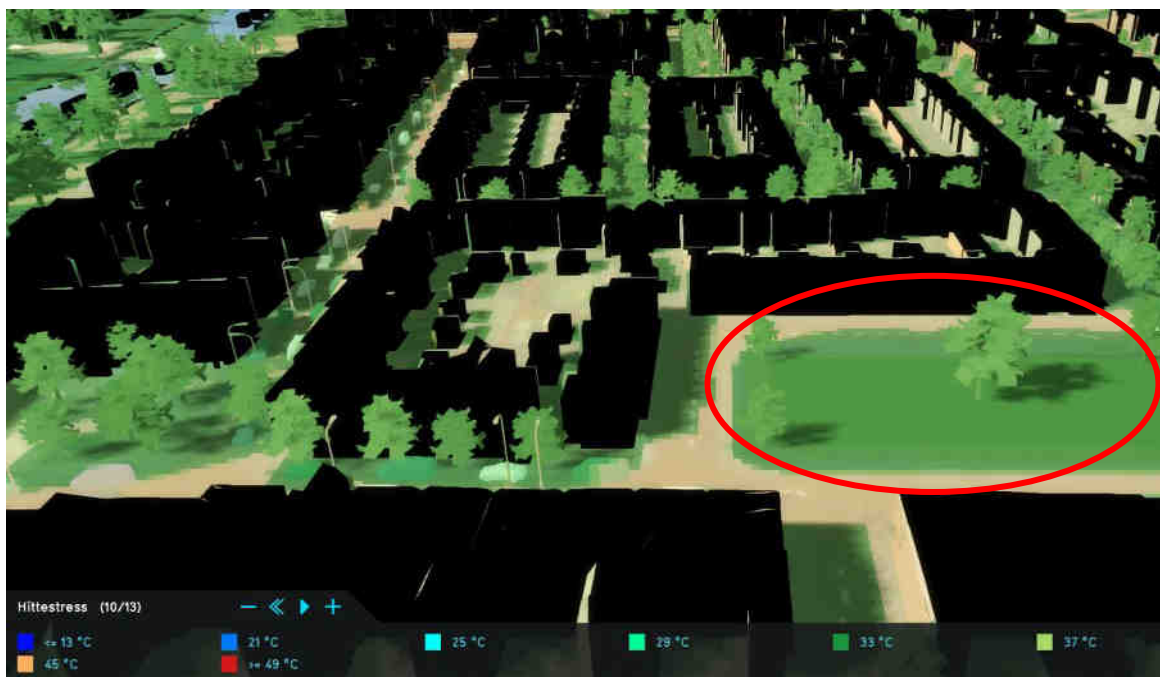
Figure 17 A close-up image at 14:00, with the Heat Overlay, for the situation with trees placed in groups, in the Rivierenwijk. The red circle shows the place where trees are added in a group (Tygron Geodesign Platform, 2020).
