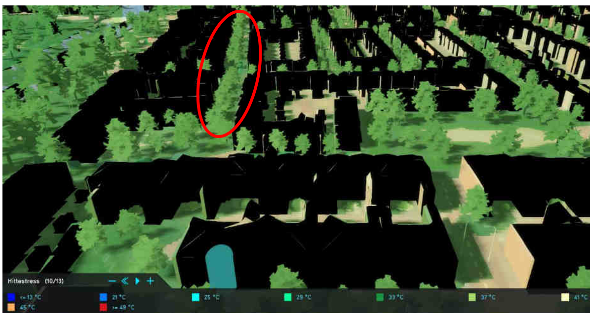
Figure 16 A close-up image at 14:00, with the DPRA Heat Module, for the situation with trees in lanes along the roads, in the Rivierenwijk. The red circle shows a street with trees, which had no trees previously (Tygron Geodesign Platform, 2020).
