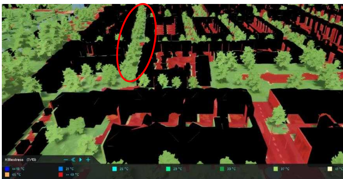
Figure 12 A close up image at 14:00, with the DPRA Heat Module, for the situation with trees in lanes along the road, in the Rivierenwijk. The red circle shows a street with trees, which had no trees previously (Tygron Geodesign Platform, 2020).
