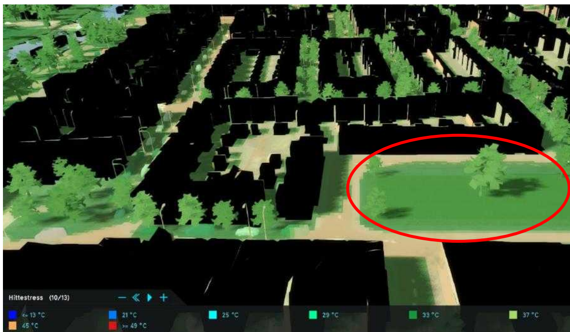
Figure 16 A close up image at 14:00, with the Heat Overlay, for the situation with trees placed in blocks, in the Rivierenwijk. The red circle shows place where trees are placed in blocks (Tygron Geodesign Platform, 2020).
